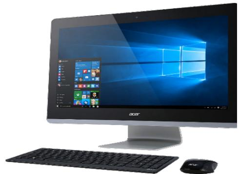
B. Desktop with Integrated System unit and Monitor
