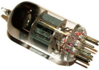
✿ **Vacuum tube** is an electronic device that controls the flow of electrons in a vacuum.
