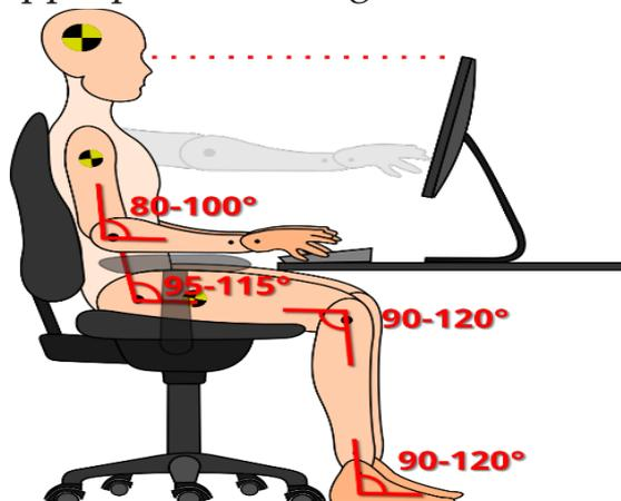
Figure 5.3. Workstation Setup
